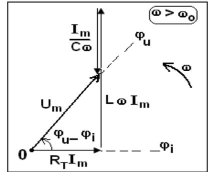
Théorème de Pythagore :  $I_m^2 [R_T^2 + (L\omega - 1/C\omega)^2] = U_m^2 \Rightarrow I_m = \frac{U_m}{\sqrt{R_T^2 + (L\omega - 1/C\omega)^2}}$  ( $I_m = U_m/Z$ )
